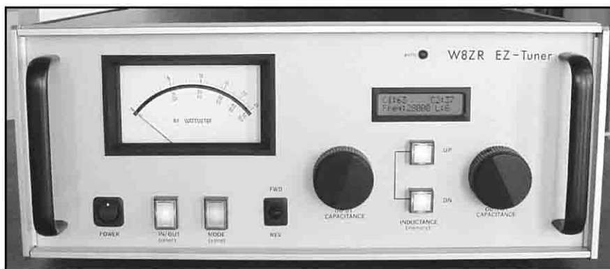
The EZ-Tuner's 16 × 7-inch brushed aluminum front panel is dominated by the large RF wattmeter. Press-on letters from an art supply store were used to label the controls. After lettering was completed, two coats of satin finish clear plastic spray sealed the panel.
